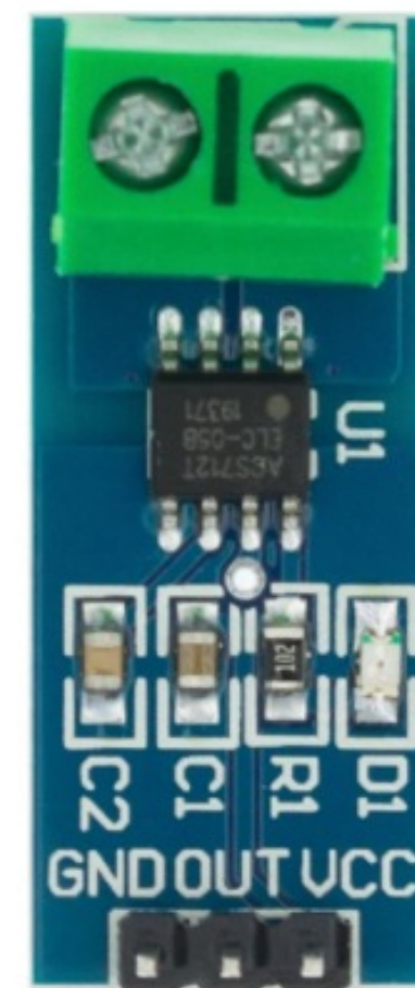
ACS712ELC 5A STROMSENSOR ANALOG CURRENT HALL SENSOR
